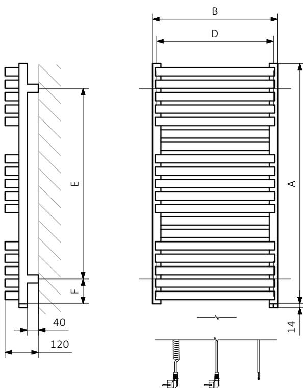
A — Height B — Width C1-C5 — Distance between pipe centres D — Horizontal distance between mounting bracket centres
