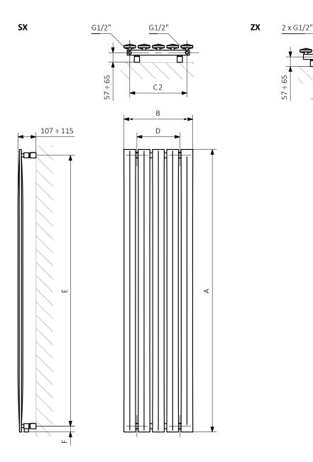
A – Height B – Width C1-C5 – Distance between pipe centres D – Horizontal distance between mounting bracket centres E – Vertical distance between mounting brackets F – Distance between a mounting bracket and the bottom of the radiator
