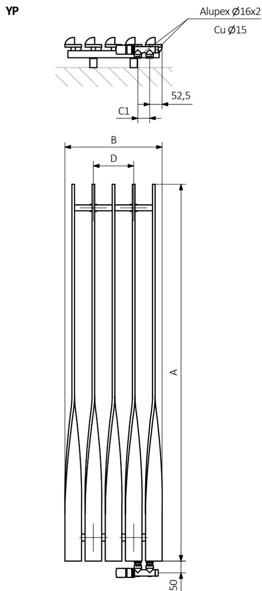
A — Height B — Width C1-C5 — Distance between pipe centres D — Horizontal distance between mounting bracket centres
