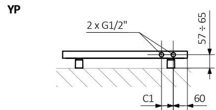
A — Height B — Width C1-C5 — Distance between pipe centres D — Horizontal distance between mounting bracket centres
