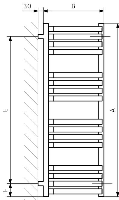
A — Height B — Width C1-C5 — Distance between pipe centres D — Horizontal distance between mounting bracket centres
